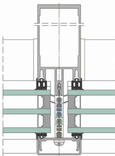
CROSS SECTION OF ANGLE STRUCTURE FA 50N
